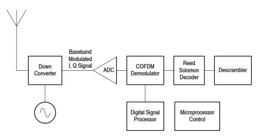
The receiver accepts a UHF, VHF or external baseband input and demodulates the COFDM signal to give an MPEG2 transport stream(s) output. The receiver operates as a stand-alone system containing an embedded controller and DSP (Digital Signal Processor), Alphanumeric display and keypad.
