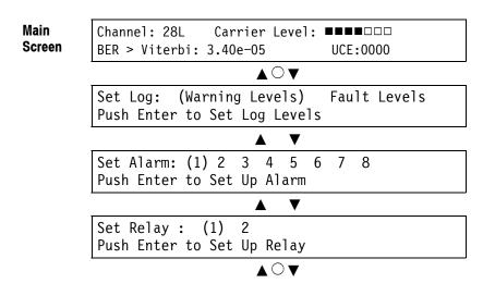
Set Log : (Warning Levels) Fault Levels Push Enter to Set Log Levels
