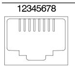
Figure C-2: Test Port Pin Numbering
