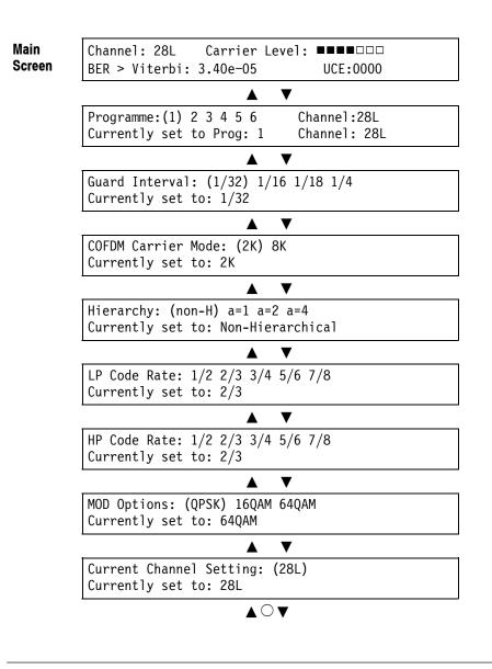
Current Channel Setting: (28L) Set to Channel: 28L
