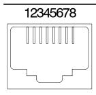
Figure C-1: Ethernet Port Pin Numbering
