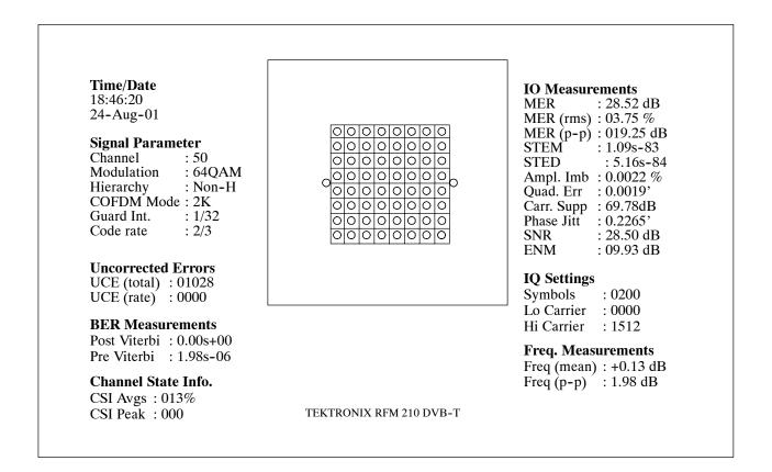
Figure 5-2: Example of output to VGA monitor
