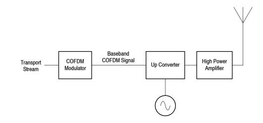
Coded Orthogonal Frequency Division Multiplexing (COFDM) is based on phase / amplitude modulation using SINE / COSINE (Orthogonal) centered carrier. The SINE / COSINE components are referred to as I / Q, (real / imaginary). This system is an adaptation of I / Q data modulation.
